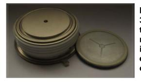
IXYS UK Westcode Ltd. introduces new 3.6kV pressure contact phase control thyristors with increased power density. The new improved design offers up to 52% increase in average current rating over the established designs, while retaining the overall package footprint.
